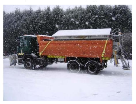
Figure 4: Demountable salt spreader
