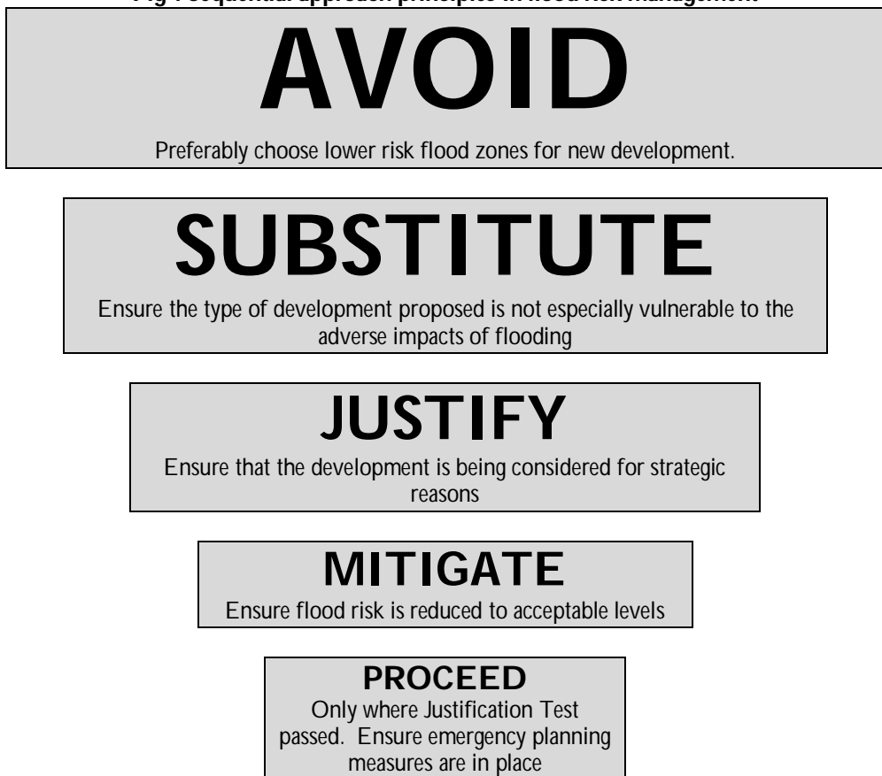
Fig 1 Sequential approach principles in flood risk management
