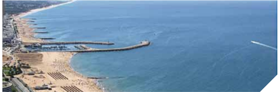
Quarteira fishing harbour and groin field, eastward of Vilamoura marine (Portugal)
