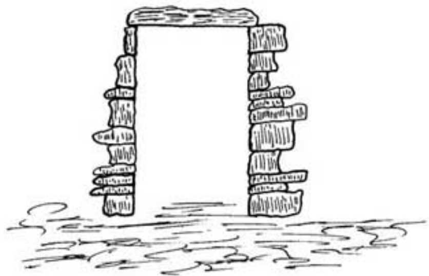
AUGHAVAL OLD CHURCH. DOOR NORTH SIDEWALL. HEIGHT 4'6". WIDTH 2'3".
