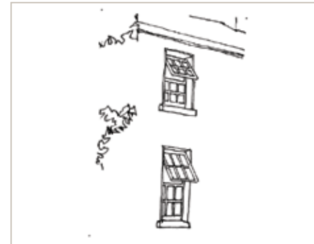
Inappropriate uPVC windows with outward openings have replaced traditional hardwood sliding sash windows. Where possible original windows and doors should be conserved or re-instated.
