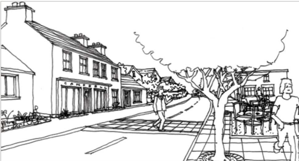
Sketch B: Proposed pedestrian crossing to promenade will slow traffic and define village centre.
